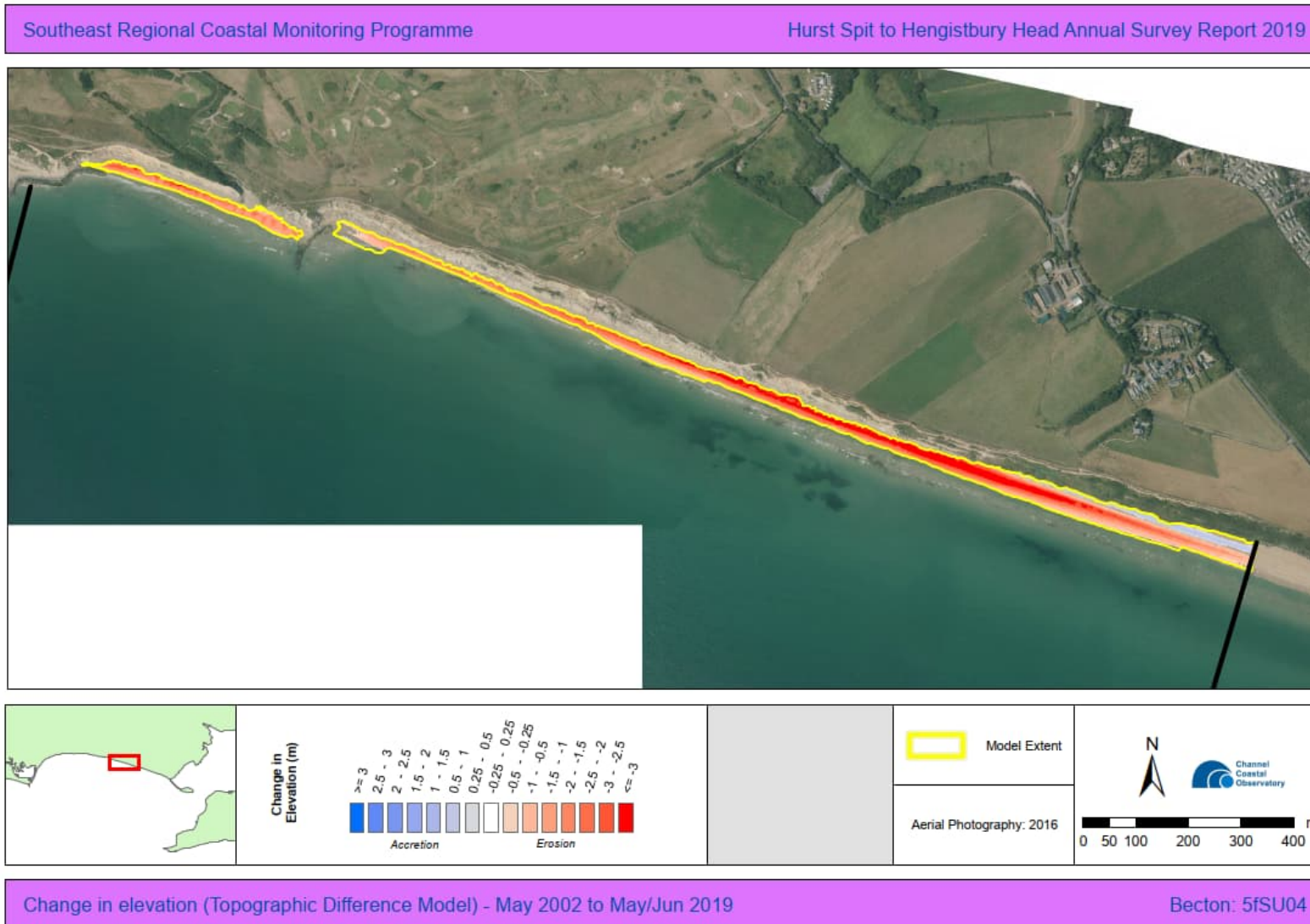
Figure 3-6: Beach profile elevation change at Becton to Hordle between May 2002 and May/June 2019. Figure obtained from the Channel Coastal Observatory (2019).
